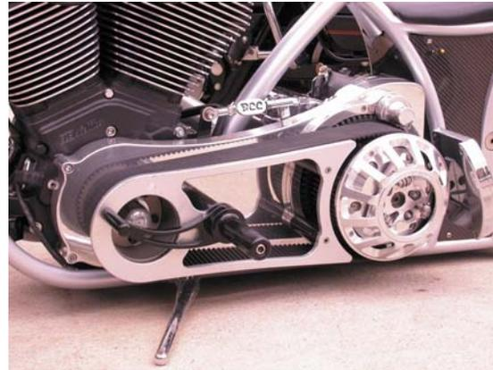
Lockup covers are available in 3 models with a bearing for use with an outboard support, and 3 models for stand alone use without a support, and will cover either a Bandit lockup or an MTC multistage lockup when used on a Bandit belt drive. Bandit belt drives are available with Tech and Primo motorplates, and are available to retrofit most other motorplates.
