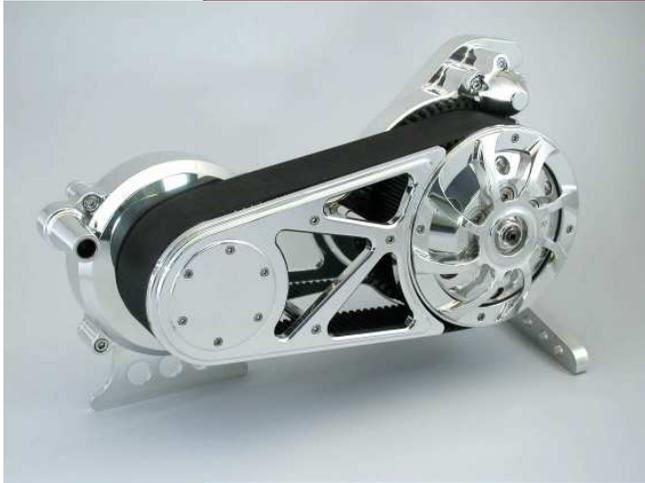
Bolt on to 1990 – 2006 Touring models, integrated shifter mount uses all stock or custom shifter components, no modifications to floorboards needed.
