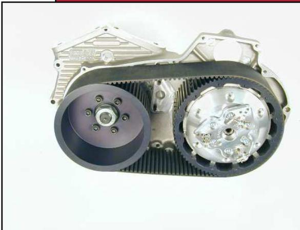
Bandit offers over 30 models of drives to fit the XL V-Twin. Varieties of belt width, lockups, ratios, etc allow for fitment to specific applications. These drives are designed specifically for the S&S 5-speed Sportster cases, adaption to stock HD cases is possible with case modification.
